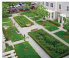
Recessed landscape for storm water capture and storage
