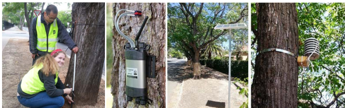
Figure 6. Flinders University researchers and PhD students installed sap flow meters in street trees to measure water use by trees with and without TREENET Inlets. Data from sensors in radiation shields (right) allow comparison of temperature and humidity in tree canopies and other street locations to quantify the cooling benefit of the additional water provided by the inlets.
