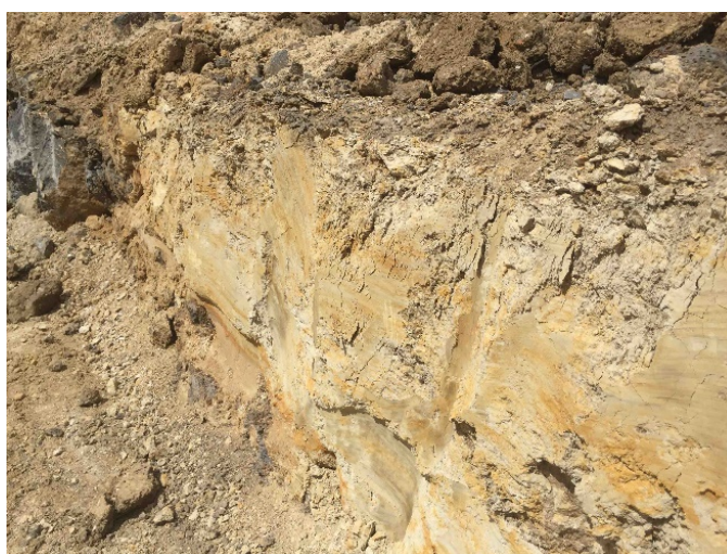
Figures 1a and 1b. Dense clay subsoils excavated for tree pits. Note the smearing of the clay (right) by the excavator bucket.
