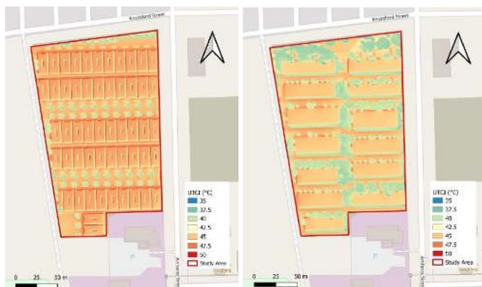
Figure 4. Modelled human thermal comfort temperatures resulting from conventional urban design (left) and cooler temperatures of WSUD and green infrastructure (from London et al. 2020)
