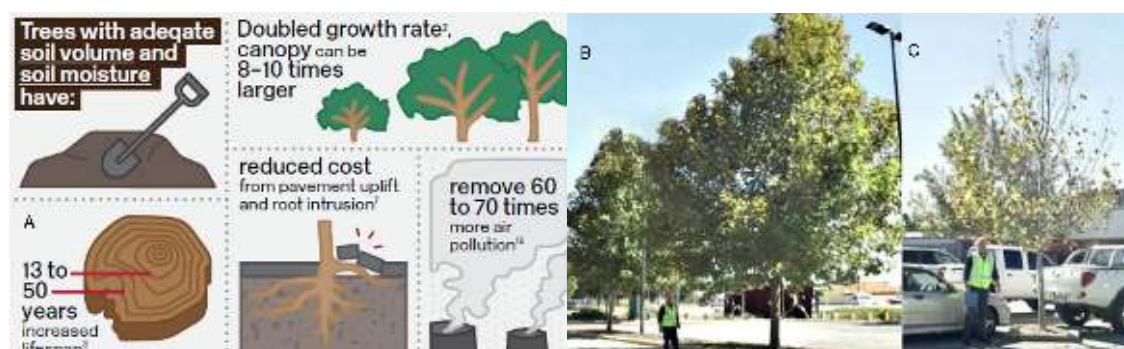
Figure 3. A: benefits of passive irrigation of trees, B: trees after 4 years growth in a car park built with structural cells, C: trees after 15 years growth in a conventionally engineered car park (Source CRCWSC, 2020).
